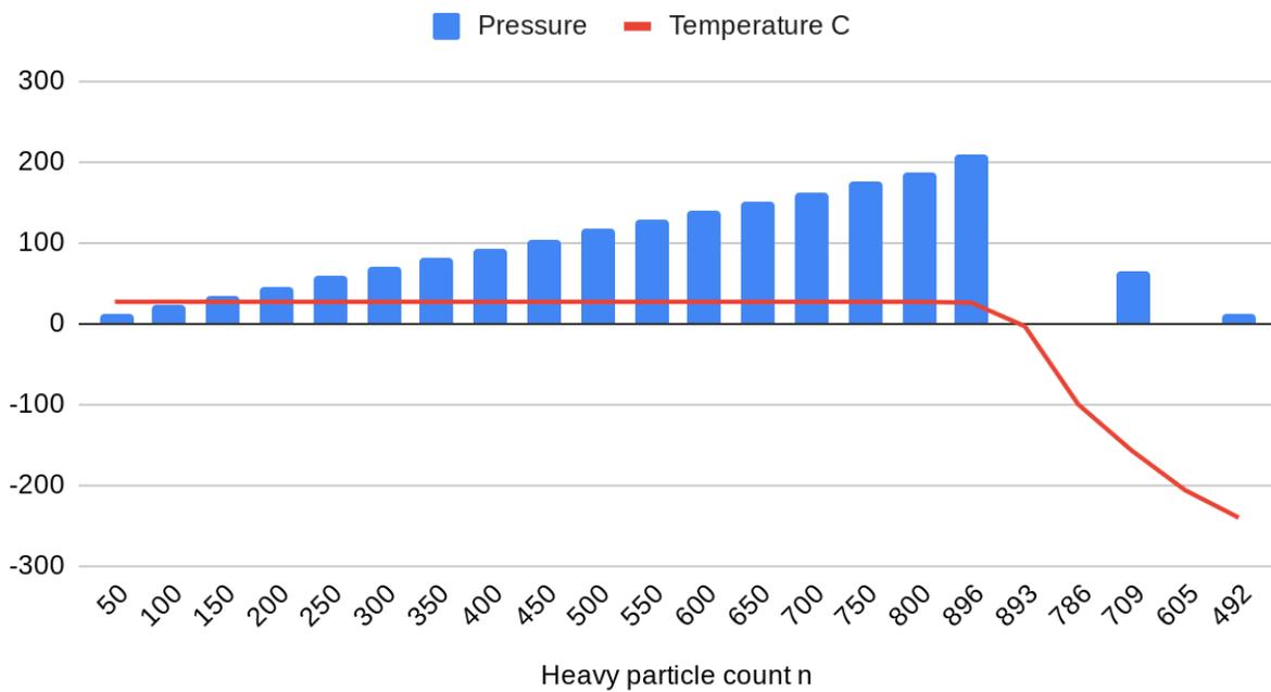
Figure 9. Graph showing that temperature dropped steeply after maximum pressure was exceed. The top of the chamber opened and gas escaped. Pressure reduced to 0.6 atm.
